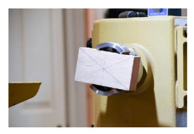
you have this you then take the marked blank and put it centered on the rectangle with two opposing jaws removed from the chuck. At this point you could use a round scrapper to make a 2" bowl that is 1" deep. However, his trick is to take a 2" Cove Box Router Bit and place it into a Jacob's chuck held in the tail
