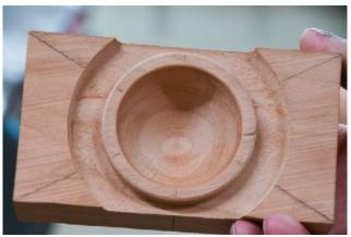
now rimmed bowl. Lightly chamfer the inside and outside of the raised rim. Sand and finish the inside of the rimmed bowl. You do this same process for the other blank. This means they will be a very precisely book-matched pair. Once these steps are done you reattach the opposing chuck jaws that were removed
