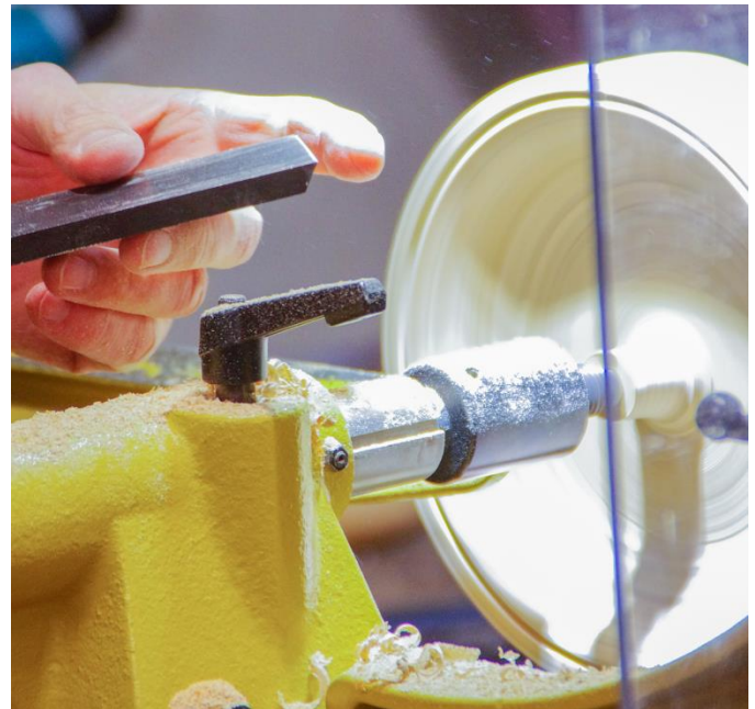
Using a heavy duty square scraper to shaped the bottom and corner of the cabinet (Note: The scraper did not have a burr, but was sharp). Also note that the center of the hollow form was left in place for. SAFETY PURPOSES
