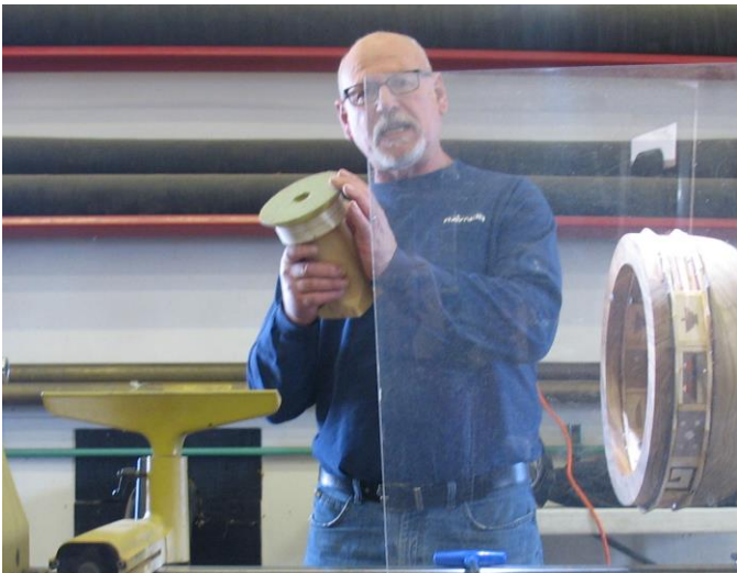
Wayne explains the Jam Chuck he created for finishing the bottom of the bowl.
