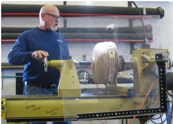
Wayne demonstrating the use of the Jam Chuck
