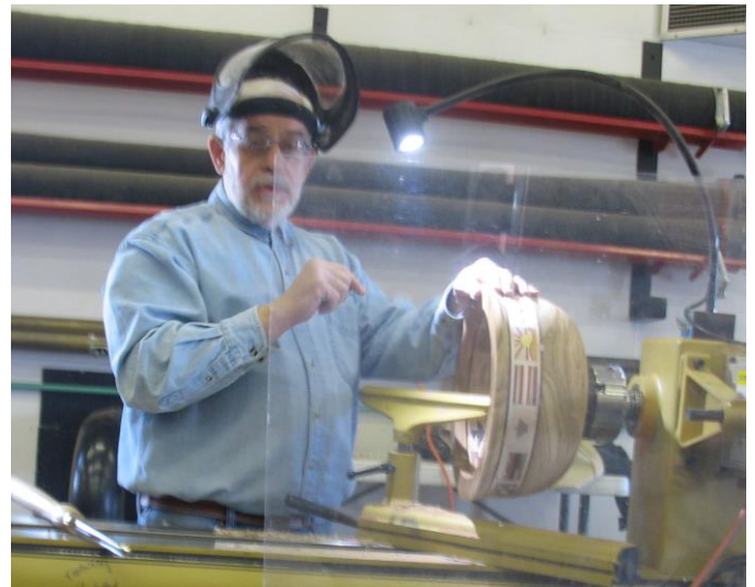
Tom then took over and started shaping the inside. His task was to shape the top where the feature ring was a challenge
