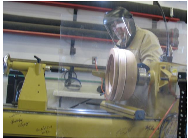
Wayne started the finish turning by shaping the outside of the bowl
