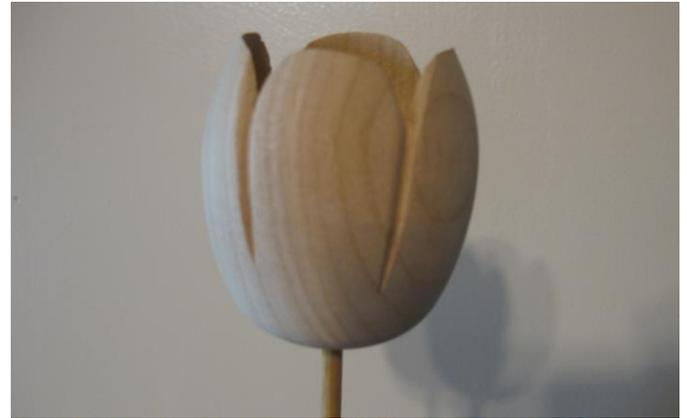
With the walls nice and thin, he then demonstrated his technique to put petal definition on the turned tulip. He used a box cutter to scribe a line and then a hand file to make the groove. A Dremel Tool can also be used to accomplish the petal definition.
