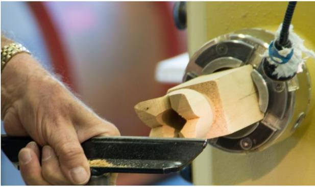
The second flower was a tulip with the petals shaped toward the center. He mounted the piece and shaped the outside and drilled the center with the Forstner Bit. He then used an Easy Wood Hollower and hollowed the inside
