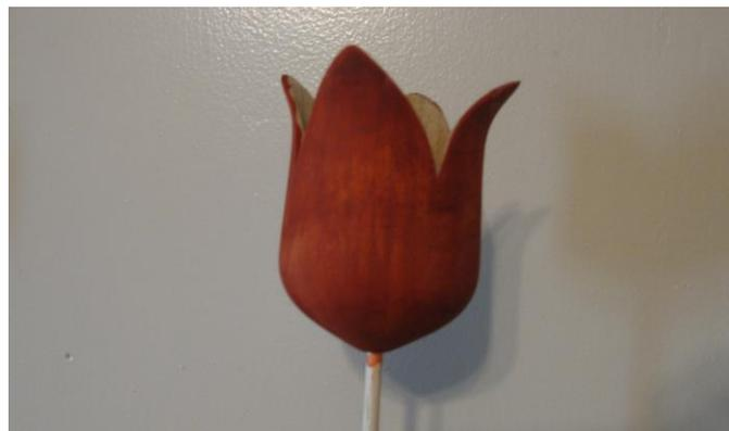
Sam showed how to mark the piece and cut out the notches with the band saw. Then he mounted the piece and shaped the outside.
